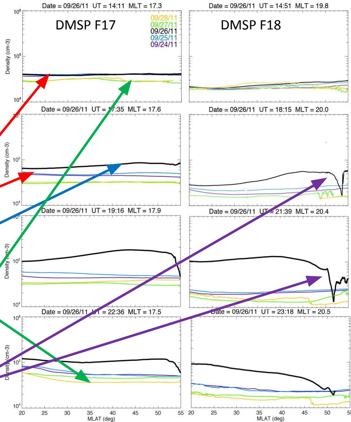
Ion density measurements from selected passes from F17 (dusk) and F18 (post dusk). Each plot shows the data for two days before and after the storm versus MLAT at similar UTs. (UT and GLON are locked for DMSP so spacecraft in similar GLON sectors at similar UTs.)
