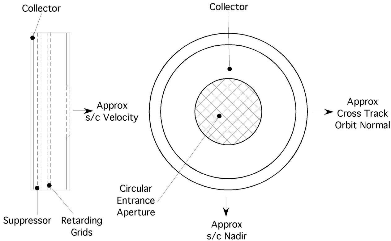
A current- voltage curve is thus produced that is a function of the retarding voltage and the collected ion current.
