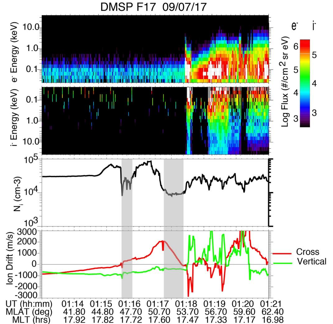
DMSP F17 measurements of the mid-latitude ionosphere trough (MIT). From top to bottom: electron energy flux, ion energy flux, ion density, horizontal and vertical ion drifts. (Adapted from Aa et al., 2017)
