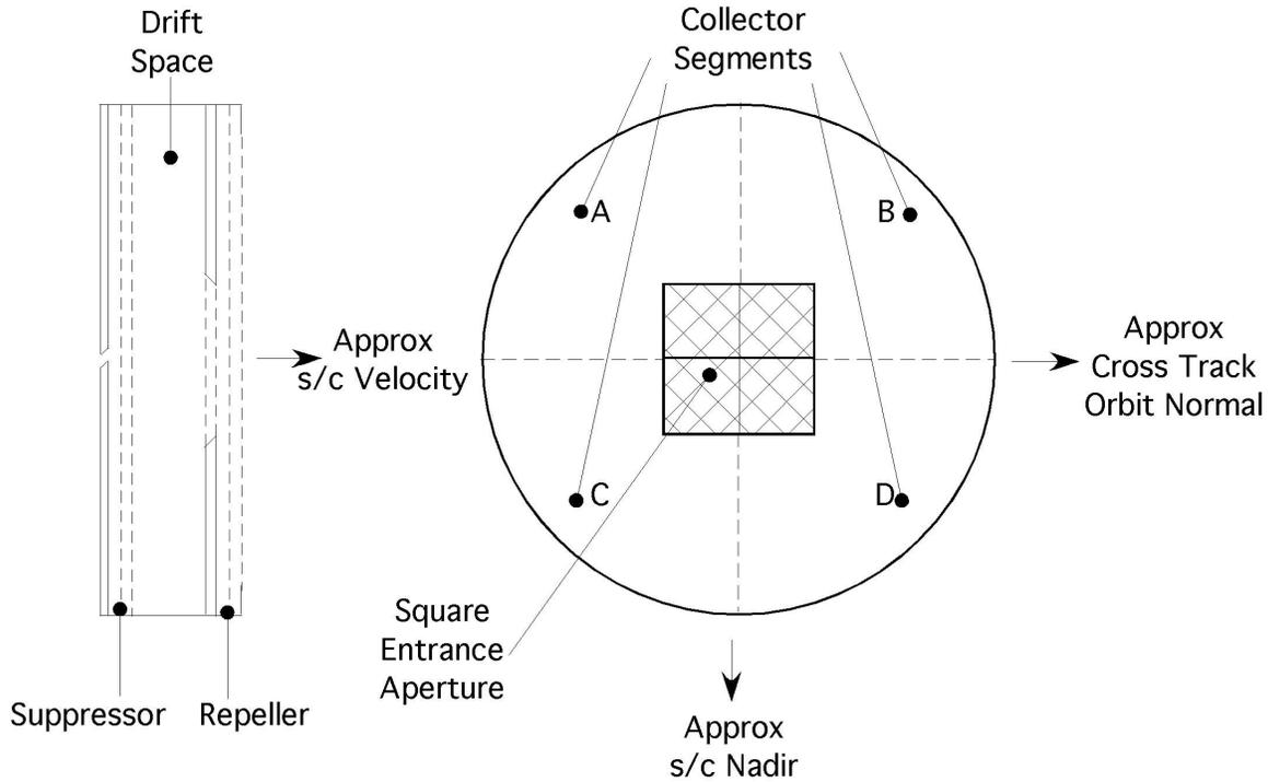
Ion beam passes through square aperture and planar grounded grids, impinges on a collector with four segments with axes parallel to the aperture edges.
