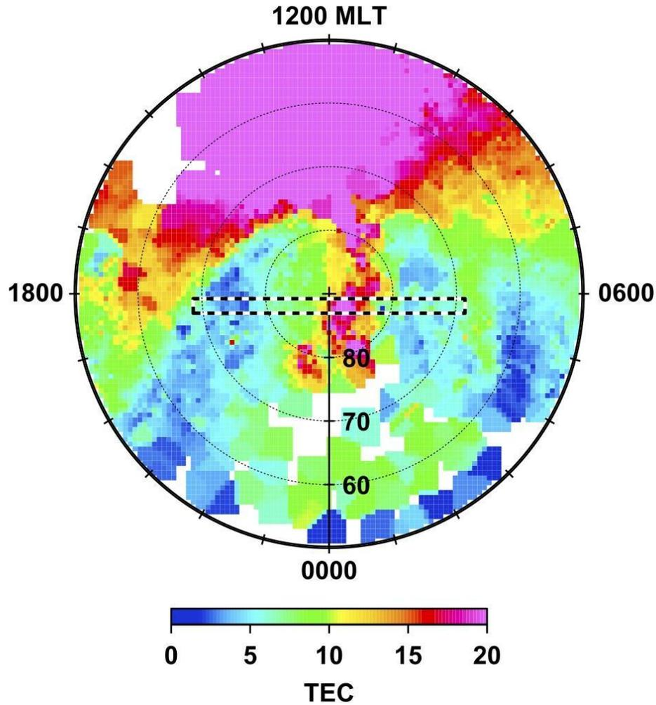
GPS TEC map in MLT (noon the top) and MLAT ( $50^\circ - 90^\circ$ ) showing a tongue of ionization (TOI) and its development into polar cap patches. [David et al., 2016]
