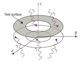
Test surfaces with horizontal orientation are placed in source region to record the counts of gamma-rays.
