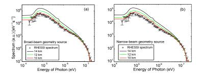
(a) The solid curves are simulated TGFs spectra at 500 km corresponding to sources with the same broad-beam geometry (isotropic within a 45° angle) positioned at different altitudes. (b) The solid curves are simulated TGF spectra at 500 km corresponding to narrow-beam geometry sources positioned at different altitudes. The RHESSI data are taken from [*Dwyer and Smith*, 2005] and the detector response matrix is taken from http://scipp.ucsc.edu/~dsmith/tgflib\_public/data/.
