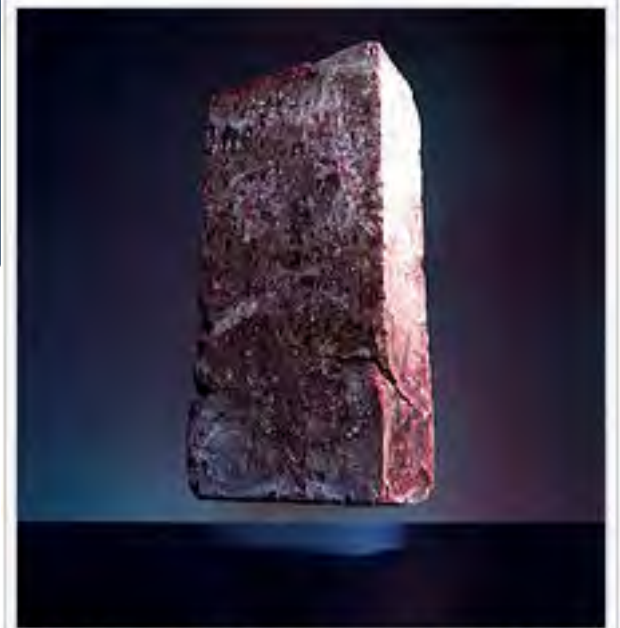
A 2.5 kg brick is supported by a piece of aerogel with a mass of only 2 grams.
