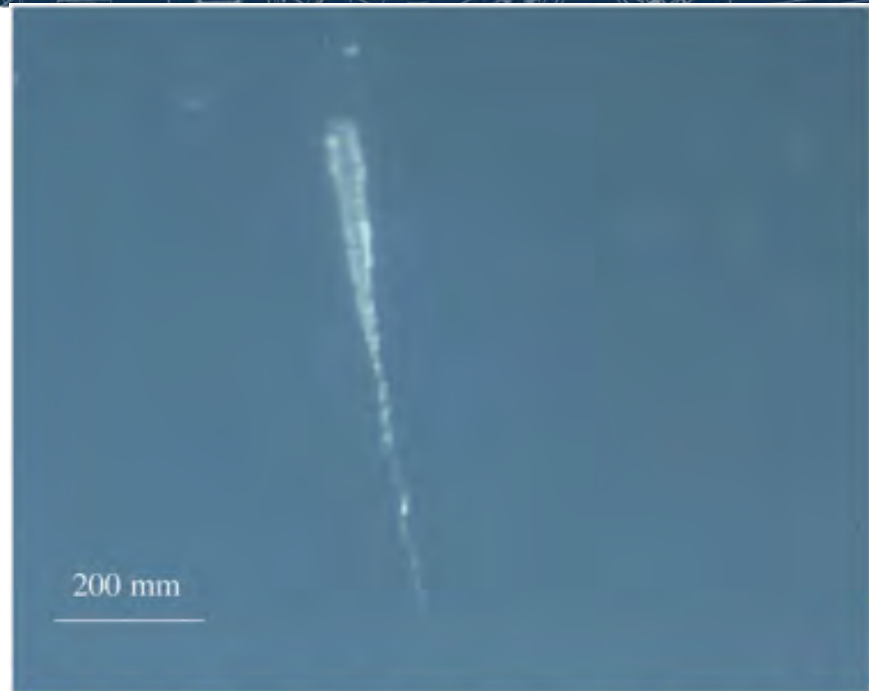
Fig. 2. Example of a Type A impact from Stardust cometary aerogel tray (Level 3 images). Typical track (C038-T7) (Burchell 2008).
