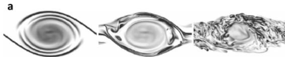
Figure: DNS results from Fritts et al. [2014] with Ri = 0.05 , Re = 2500 evolution in 0.5 T_b .
