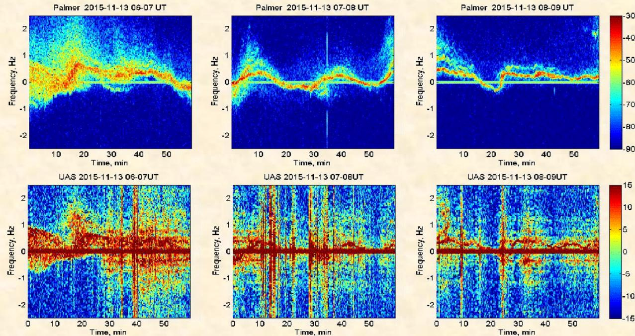
Spectrogram of HF signal ( $f_w = 5.555$  MHz) recorded at Palmer (upper panel) and UAS (lower panel) stations on 2015.11.13, 6:00-9:00 UT.
