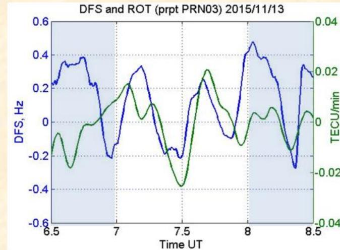
Variations of DFS (blue line) of HF signal received at Palmer station on 2015.11.13 at 6:30-8:30 UT and the rate of change of detrended TEC for GPS satellite PRN03 obtained at PRPT stations
