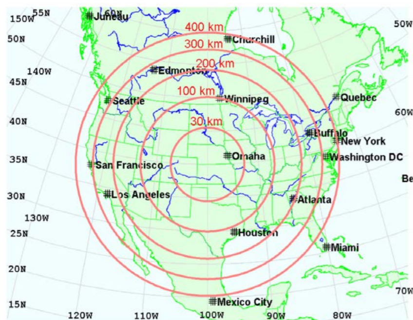
Fig. 7 Samples of E1 HEMP exposed regions for several burst heights. The red circles show the exposed regions for the given burst heights, for a nuclear burst over the central US (from Savage et al. 2010)
