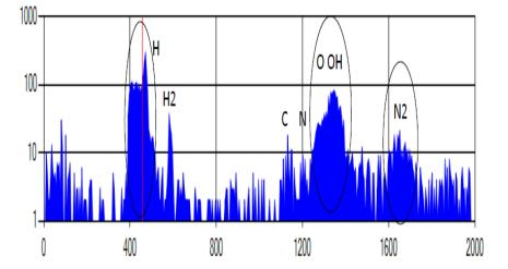
On-orbit INMS neutral spectrum – of outgassing From the instrument, only. Ram direction atmospheric sampling will produce signals 10^5 times greater.
