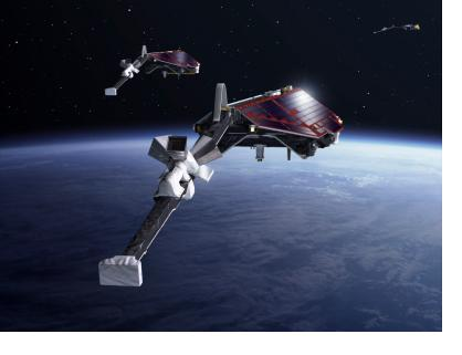
Swarm is the fifth Earth Explorer mission approved in ESA's Living Planet Programme. Three Swarm satellites with identical instruments orbit the Earth at altitudes between 460 and 530 km, measuring **E**, **B**, Te,Ti, Ne etc...
