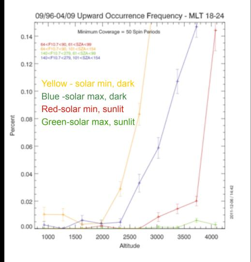
Expanded scale shows altitude where beams are first seen increases with increasing solar flux:
