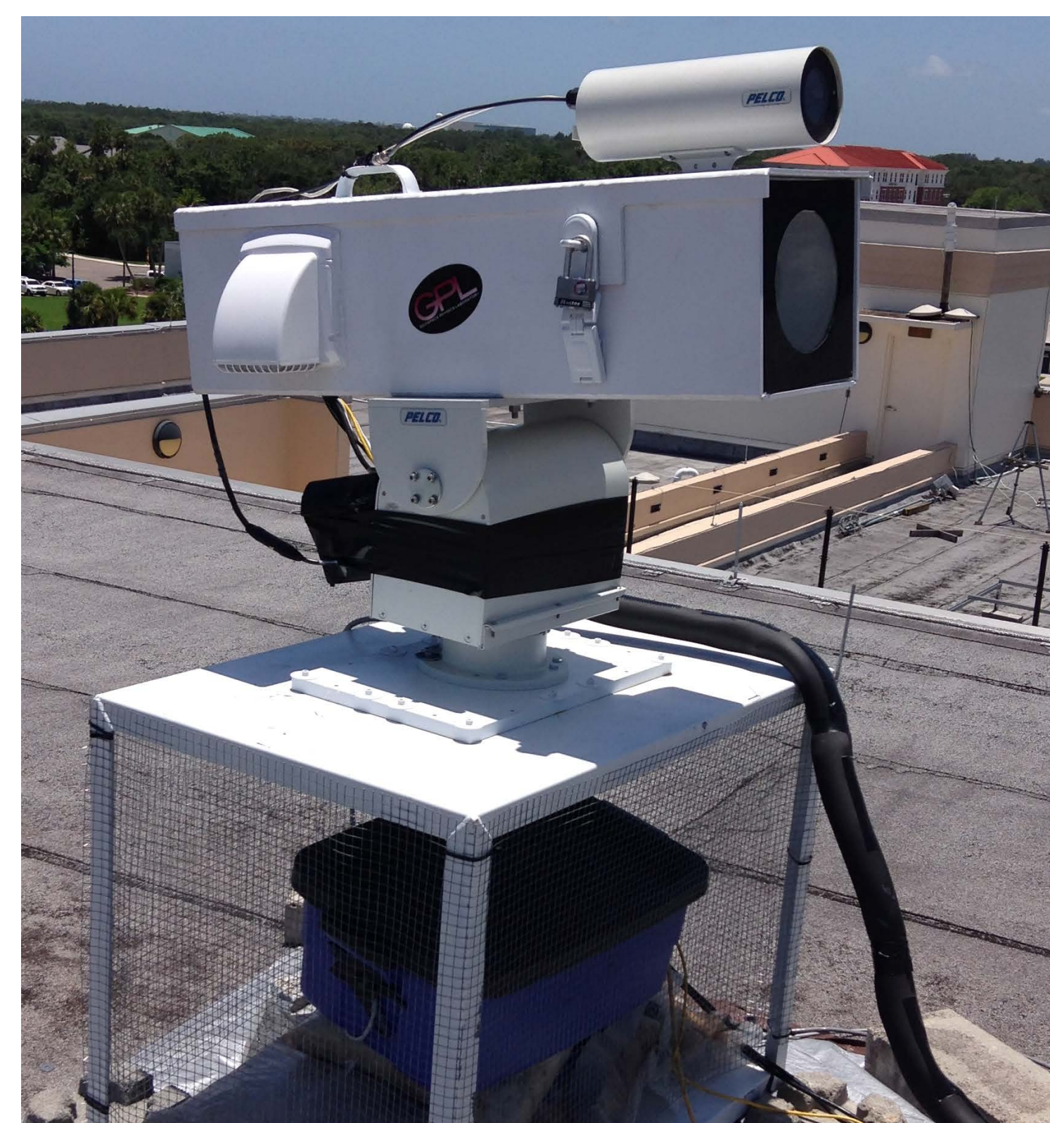
Figure 1. Finished spectrograph system with enclosure, mounted on a heavy duty Pelco motor.
