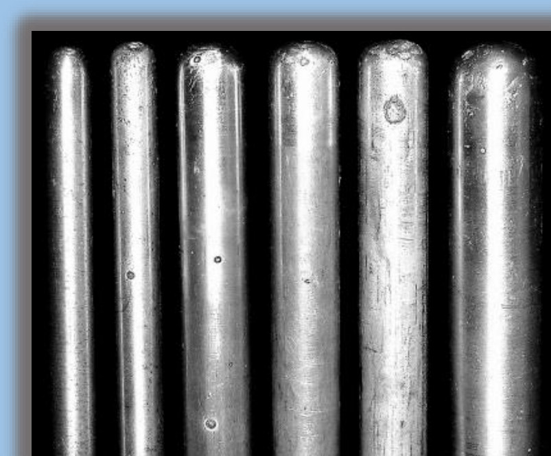
Figure 4: Photograph of six blunt aluminum rods, each of which has been struck by lightning on South Baldy Peak (Moore et al., 2003).
