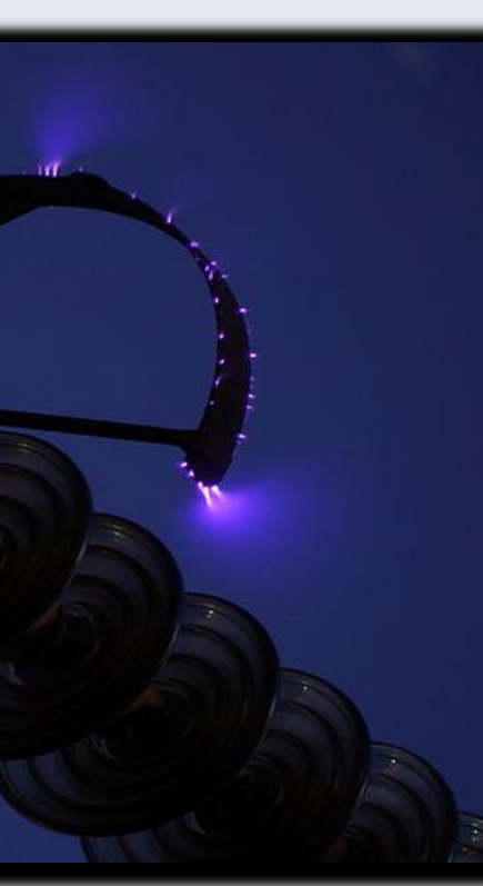
Figure 1: Glow Coronas form on the edges of a powerline transformer (Berkoff, 2005).
