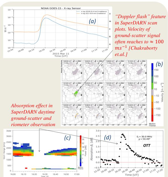
Figure 1: Typical solar flare event and its impacts on various HF systems: (a) GOES-15 X-ray sensor data, (b) FoV Doppler velocity scan plots for m SuperDARN Blackstone radar, (c) SuperDARN (Blackstone, beam 7) received power response during solar flare, (d) riometer (Ottawa station) response (HF absorption) to the solar flare.
