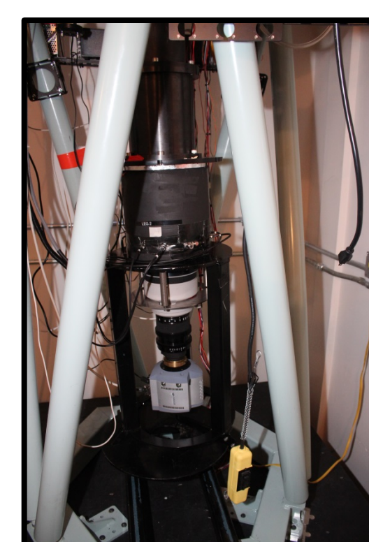
Figure 5: Close up of the main optical assembly of the South Pole instrument. This view shows the etalon chamber, the (rare and expensive) Nikkor 300 mm f/2 fringe forming lens, and the Andor EMCCD camera. Photo taken by Dale Pomraning
