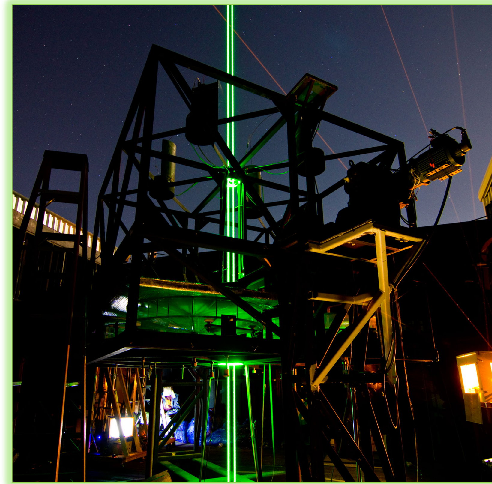
Figure 1: Large telescope system. The four 1.25 m mirrors are mounted in the cage where the two laser beams pass through the center of the cage.
