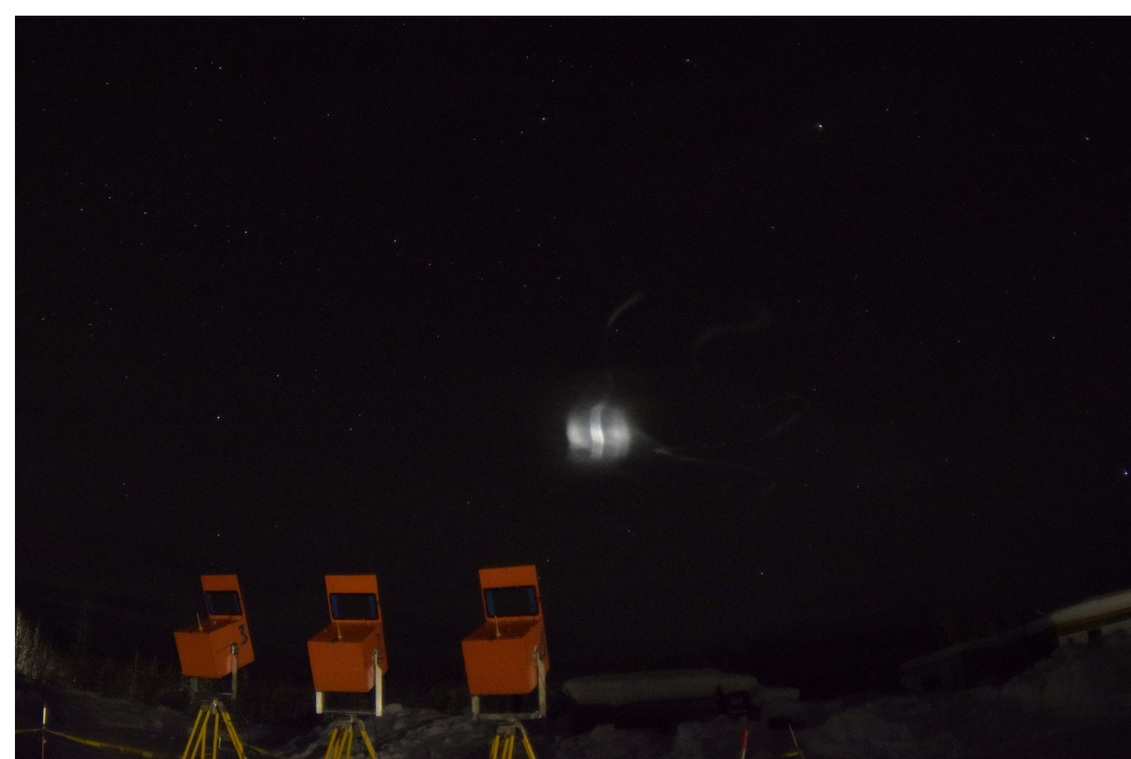
Figure 1: Camera setup from Coldfoot/AK with the TMA releases on the background.
