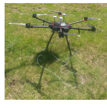
UAV drone used for antenna pattern measurement
