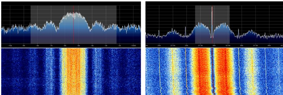
Figure 1. Inmarsat downlink signal (left) and SARSAT downlink signal (right)
