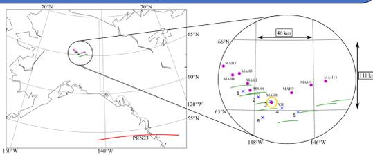
Figure 1: The Mahali GPS receiver array (magenta dots) in Alaska with PFRR all-sky camera and PFISR (yellow circle). PFISR beams (blue crosses) at the mapping altitude are shown with the GPS receiver-satellite lines-of-sight (green lines).
