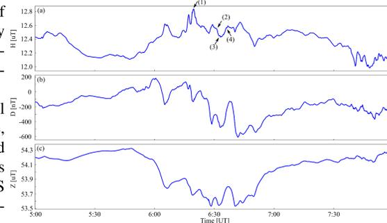
Figure 2: Magnetogram (variations in HDZ components) from the PFRR fluxgate magnetometer for the event. Enumerated events within the dashed lines marks the six successive passages of the WTS. Enumerated are four events presented below.
