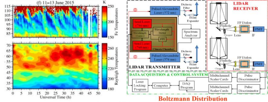
A lidar campaign ongoing at McMurdo (77.84°S, 166.67°E), Antarctica has been provided 9 years of high-resolution temperature data from 30 to 115 km. The Fe Boltzmann lidar measures iron (Fe) layers, atmos. density, aerosol layers, and temperatures [Chu et al., 2011; Chen et al., 2016].
