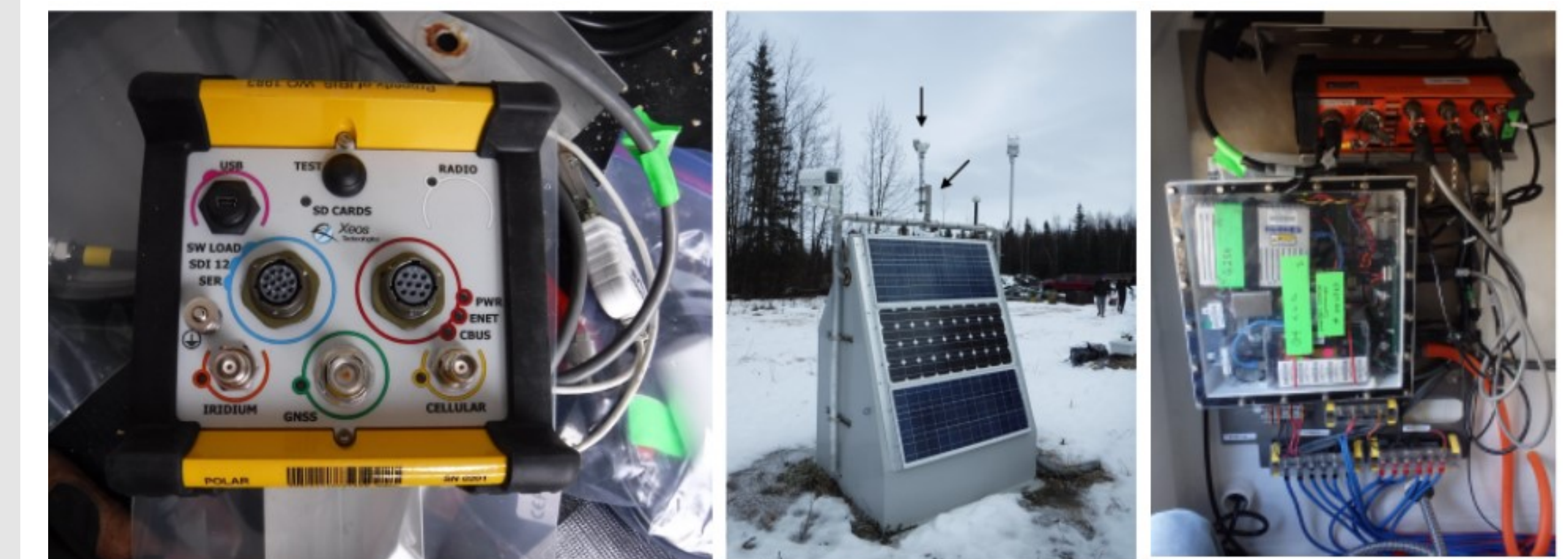
Figure 9. (left) The Xeos Resolute Polar unit pictured above was installed at the Alaska TA station O22K on 31 January 2019. (center) Alaska TA station O22K is an autonomous, telemetered station installed in Cooper Landing, Alaska. The GNSS antenna was added to the existing station mount (arrows), which holds the communications equipment and meteorological sensor. (right) hut interior showing electronics package.
