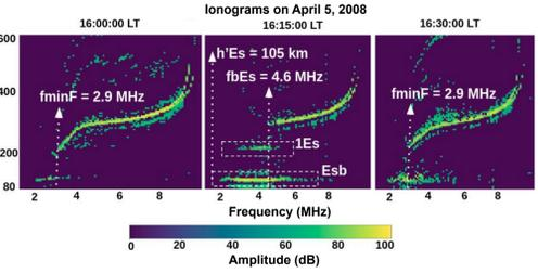
Figure 2. Parameters of Esb in ionograms
