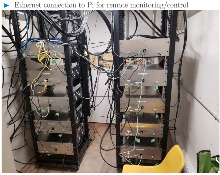
► Similar setup to receiver system ▶ X300 transceivers on rack connected to 10 Gbps Switch
