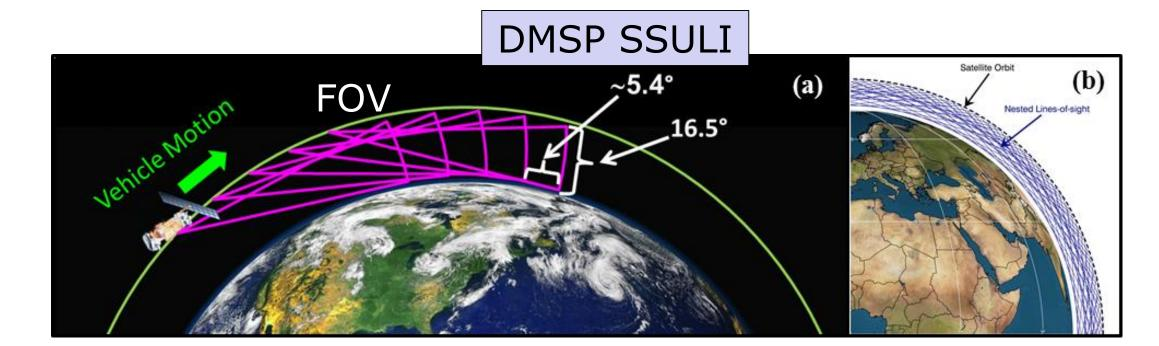
SSULI is a UV spectrograph on DMSP, oriented to view the limb along the orbital track every 92 sec
