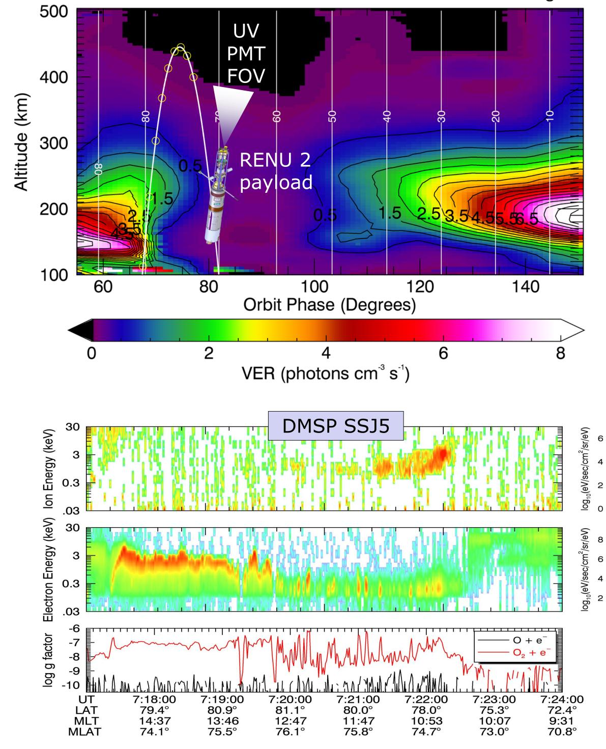
SSULI intensity measurements  $(I_{1356})$  are used to reconstruct volume emission rates  $(\varepsilon_0)$  through an inversion process.
