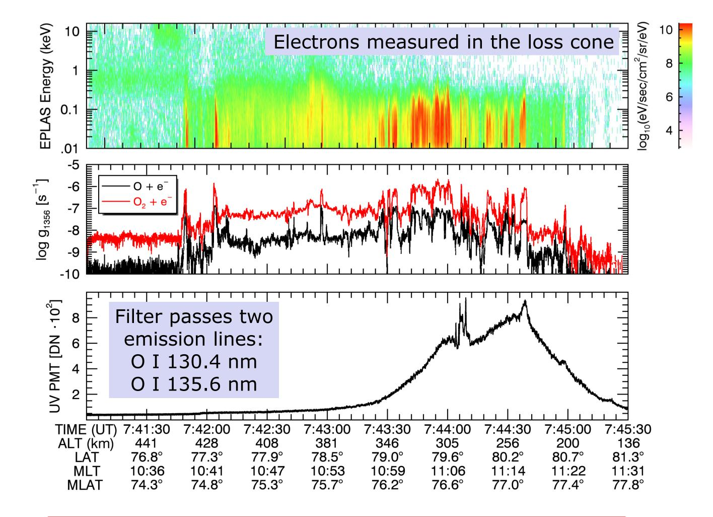
Electron collisions are the main source of O I ( $\lambda$  = 135.6 nm) production. The RENU 2 EPLAS instrument measured electron flux,  $\varphi(E)$ . Excited state oxygen atoms, 0<sup>\*</sup>, emit photons from several reactions, including:
