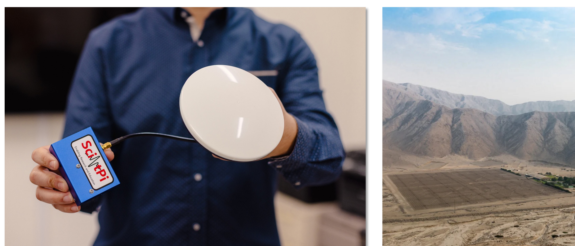
Figure 1. (Left) Team member holding a ScintPi 3.0 scintillation monitor [2] used in this project. Cost of parts including antenna: ~600 USD. (Right) View of the Jicamarca Radio Observatory in Peru where the real-time system was implemented and tested.
