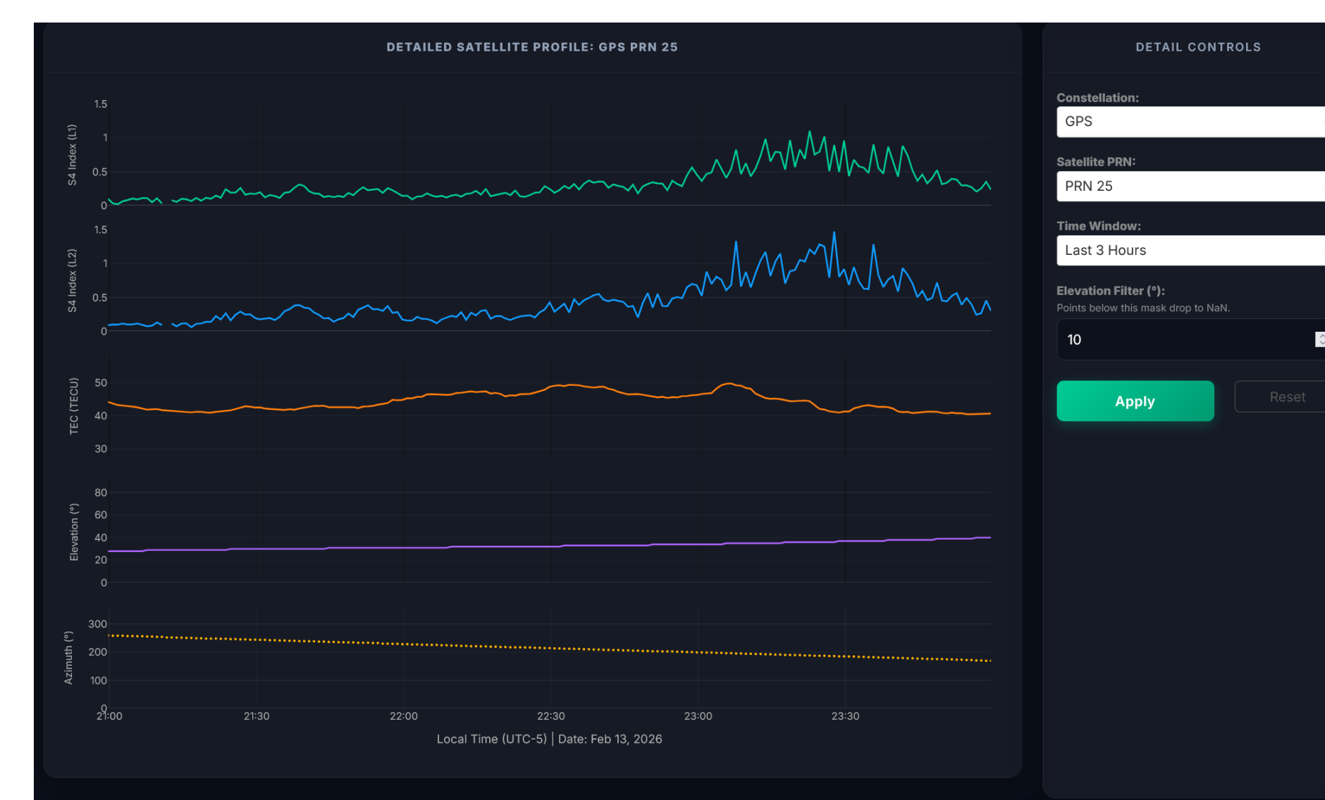
Figure 4. Example of the second panel that forms the web-based dashboard. It shows the current and previous several hours of measurements made using signals from GPS PRN 25. From top to bottom: L1 S_4 , L2 S_4 , slant TEC (1 TECU = 1 TEC Unit = 1 \times 10^{16} electrons/m 2 ), elevation, and azimuth. The control panel on the right allows the user to select a specific satellite, time window, and elevation mask.
