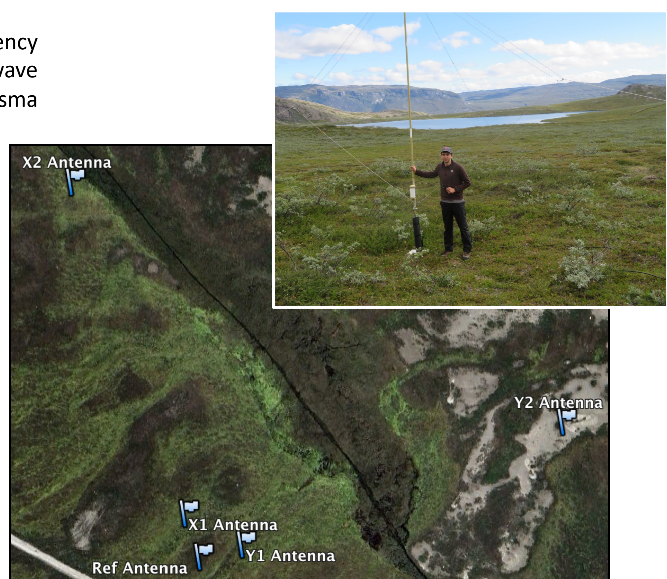
Figure 7: DOA data were collected with a 5-antenna array in Sondrestrom, Greenland (73.3° magnetic latitude). The larger array is used for the higher frequency channels (850–3100 kHz), and the smaller array is used for the lower frequency channel (100–850 kHz). Both arrays share the reference antenna shown.
