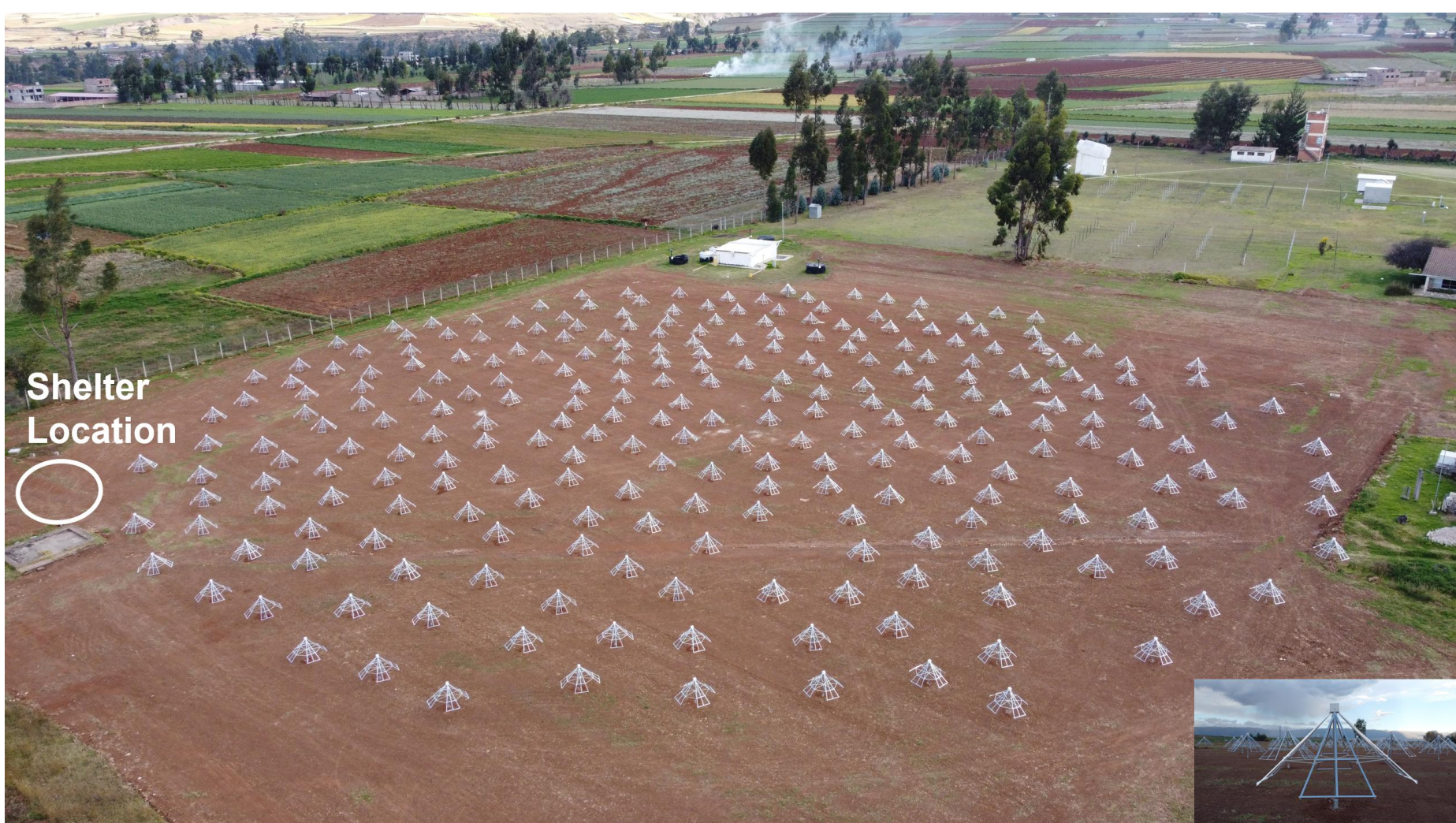
Figure 2. Aerial view of the LWA antennas deployed in Huancayo, Peru. A shelter enclosure will be deployed in the circled area to house the electronics comprising the analog and Digital Signal Processing (DSP) pipeline for J-ARGUS.
