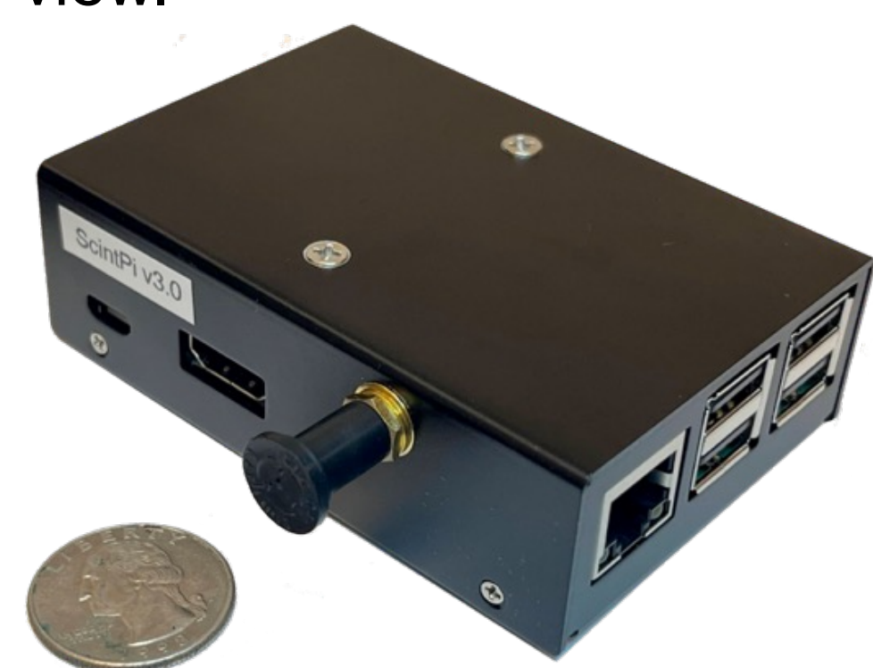
Figure 1. ScintPi 3.0 scintillation monitor [1] used in this project. Cost of parts: ~600 USD.
