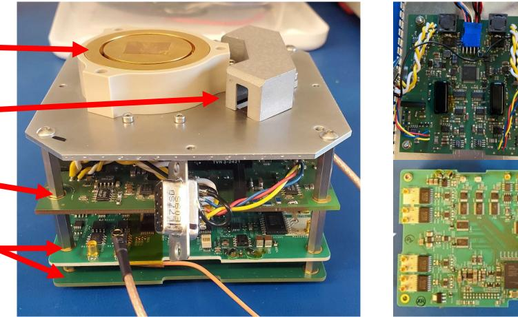
Left: Assembled SWARM-EX Instrument Deck EDL Right: (Top) FIPEX EDU Electronics Board, (Bottom) I-SENSE EDU Science Board
