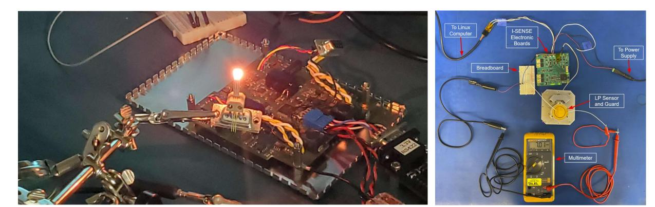
Left: FIPEX Sensor heating up during MCT Right: I-SENSE Langmuir Probe MCT testing settup
