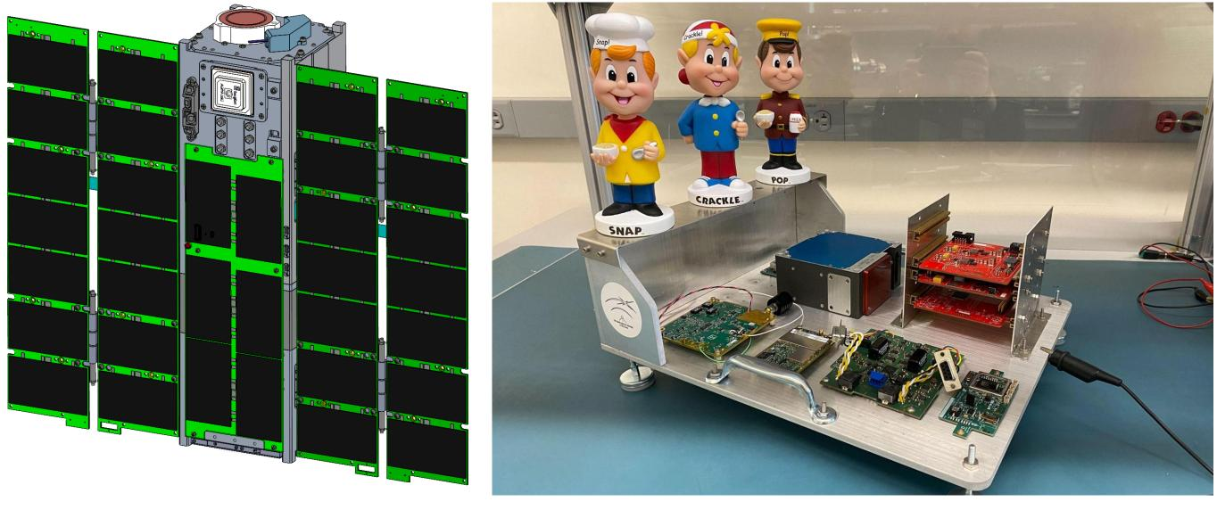
Left: CAD render of the integrated SWARM-EX satellite with solar panels deployed RIght: Assembled SWARM-EX FlatSat
