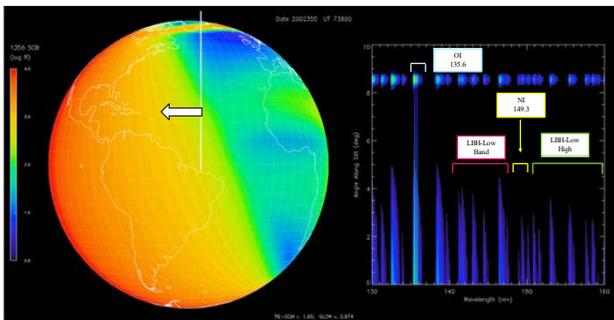
Shown here is an illustration of typical GOLD OI emission data and the swathing direction. On the right is a display of the emission spectrum obtained along the slit. Image courtesy of S. Solomon.
