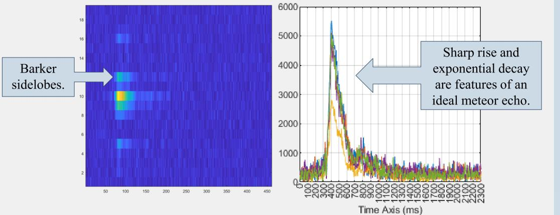
A meteor as detected by the SKiYMET radar in Puerto Rico.
