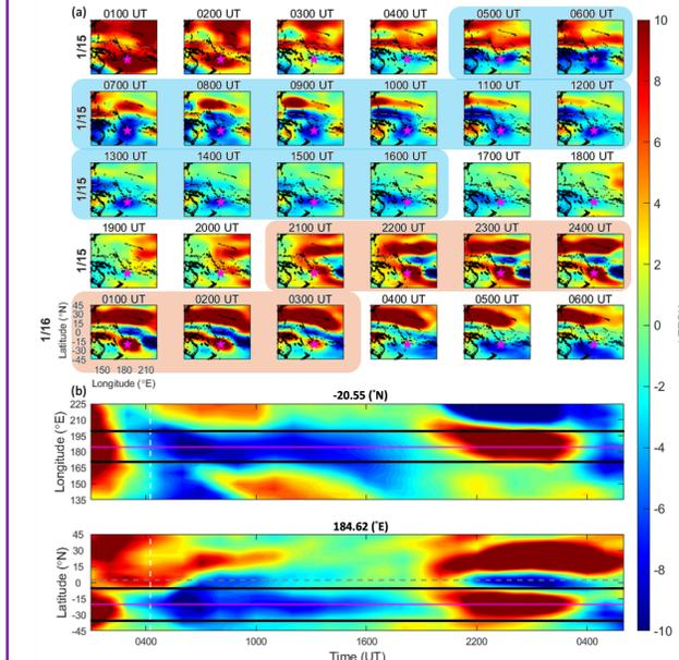
Fig. 3 Difference in GIM TEC between the observation day and the background near the Tonga volcano from 1800 UT on 14 January 2022 to 0600 UT on 16 January 2022. (a) Hourly TEC variation within the study region (135°E to 225°E, 45°S to 45°N). (b) TEC variation at a longitude of 184.62°E and latitude of -20.55°N.
