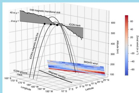
**Fig. 2** Diagram showing how ICON supports simultaneous observations of lower thermospheric winds and ionospheric plasma velocities (Immel et al 2021)
