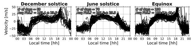
Figure 5. Daily mean vertical plasma drift curves from MP ISR observations sorted by season. Panels are annotated with the number of observations in each season and the average daily F10.7 solar flux index in solar flux units, as well as the F10.7 standard deviation.
