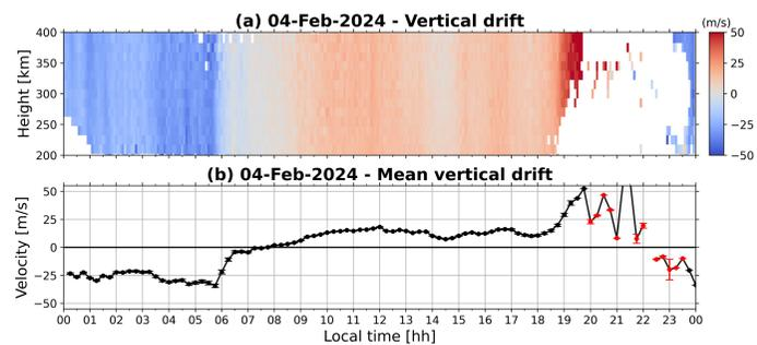
Figure 3. (a) Vertical plasma drifts at ionospheric F-region heights and (b) corresponding mean drift values for MP ISR observations on 4 Feb. 2024. 15-minute weighted averages (i.e., inverse-variance weighted means) were computed to obtain values. Values plotted in red indicate 15-minute bins with < 15 available F-region drift measurements due to ESF.
