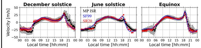
Figure 7. Quiet time drifts reproduced from MP ISR (black) analyses, SF99 model (blue), and SR20 model (red). Inputs to the SF99 model are local time and F10.7. Inputs to the SR20 model are local time, F10.7, and height (350 km).
