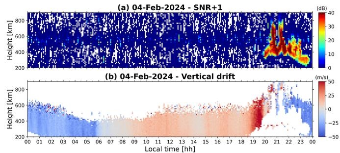
Figure 2. (a) Range-Time-Intensity map of MP ISR coherent echoes and (b) vertical plasma drift estimates for 4 February 2024.
