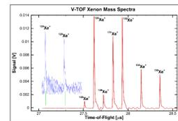
View of the Xenon isotopes recorded by V-TOF-MS. Blue inset shows further zoom-in of <sup>124</sup>Xe<sup>+</sup> and <sup>126</sup>Xe<sup>+</sup> isotopes showcasing dynamic range.
