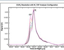
TOF spectra displaying doublet of CO<sup>+</sup> (27.99435 u) and N<sub>2</sub><sup>+</sup> (28.0055 u) as measured by the W-TOF MS.
