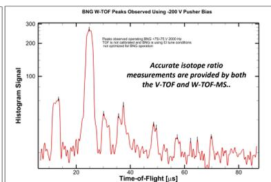
Plot at right showing first TOF spectrum obtained with BNG operation. Ions created with small ion source and gated into W-TOF-MS with BNG. Further optimization for improved performance is underway.
