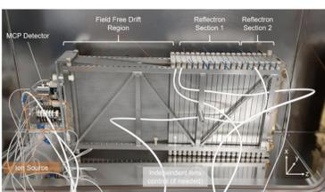
Photograph of V-TOF-MS with labeled components in the TOF development vacuum chamber.
