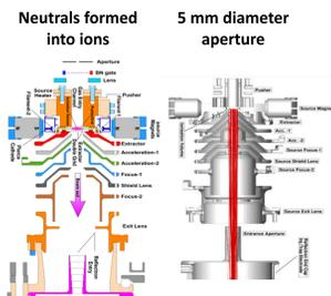
MSTR Electron ionization storage time-of-flight source with simulated ion trajectories. Left panel shows relative position of the aperture and BN gate. The gas entry channel allows direct entry to the ionization region.
