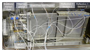
Photograph of W-TOF-MS and Bradbury-Nielsen gate (BNG) incorporated on the neutral ion source currently under development.
