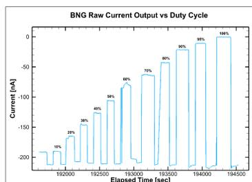
Left plot shows operation of BNG at various duty cycles. At 100% duty cycle (Gate Closed), no measured ion current. At 0% duty cycle, maximum ion current achieved. Duty cycle incremental steps investigated.
