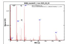
Mass spectrum of noble gas mixture – He, Ne, Ar, Kr, Xe – recorded by V-TOF-MS.
