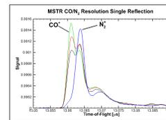
TOF spectra displaying doublet of CO<sup>+</sup> (27.99435 u) and N<sub>2</sub><sup>+</sup> (28.0055 u) measured by V-TOF MS.
