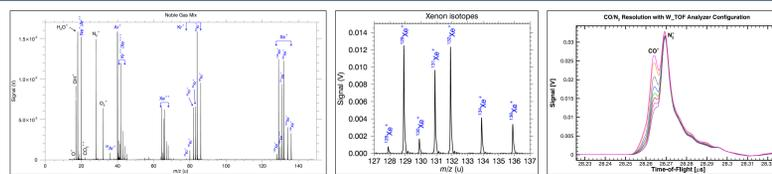
Mass spectrum of a noble gas mixture – He, Ne, Ar, Kr, Xe – recorded by W-TOF-MS. Noble gas ion signals labeled in blue, background residual gas labeled in black.
