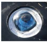
Figure 1: OH IR (0.9-1.7μm) all-sky airglow imager.
