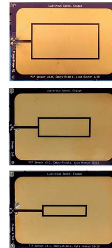
Figure 5: From top to bottom, the Large, Medium, and Small plates
