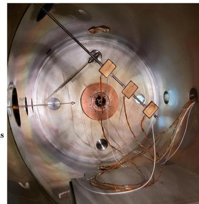
Figure 7: Image of three planar probes in the LPC, each spaced 8cm from each other
