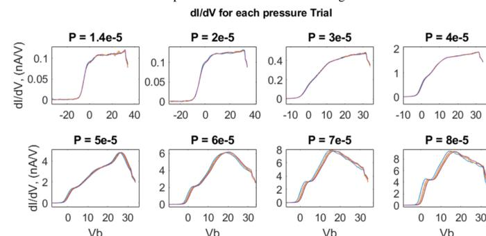
Figure 9: First derivatives of large plate IV curves, all upsweeps shown
