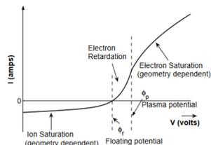
Figure 1: Langmuir Probe IV Curve
