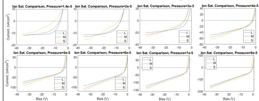
Figure 10: Ion Saturation regions for each pressure, each plate type overlaid
