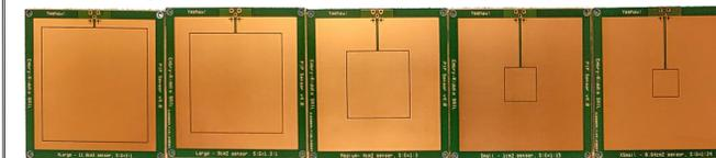
Figure 6: A set of new square plates with guard thicknesses from 1.7cm to 2mm
