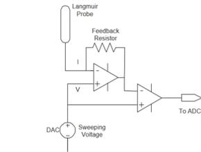
Figure 2: Langmuir Probe Electrometer circuit
