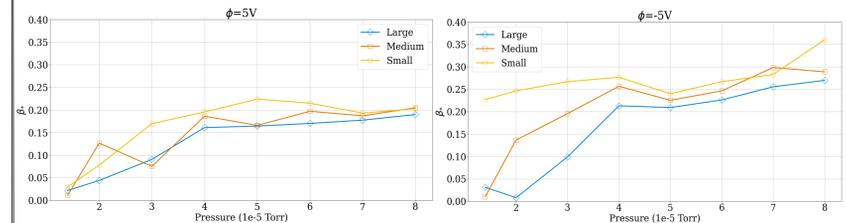
Figure 11: Pseudo-Beta plots for different comparison voltages
