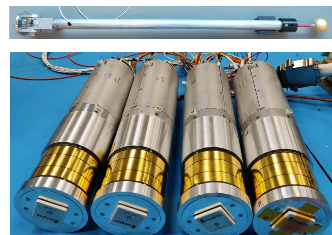
Figure 3: (Above) Main payload gold-plated, spherical PIP sensor on deployable boom. (Below) ROB ejectable subpayloads. Gold, cylindrical sensor.
