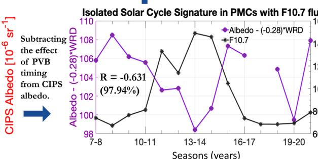
Fig 4.  $Albedo_{CIPS} - (-0.28 \cdot WRD)$  instead of being a straight line from Eq. 1, is anticorrelated with F10.7 cm solar flux. By subtracting the PVB effect from CIPS albedo.
