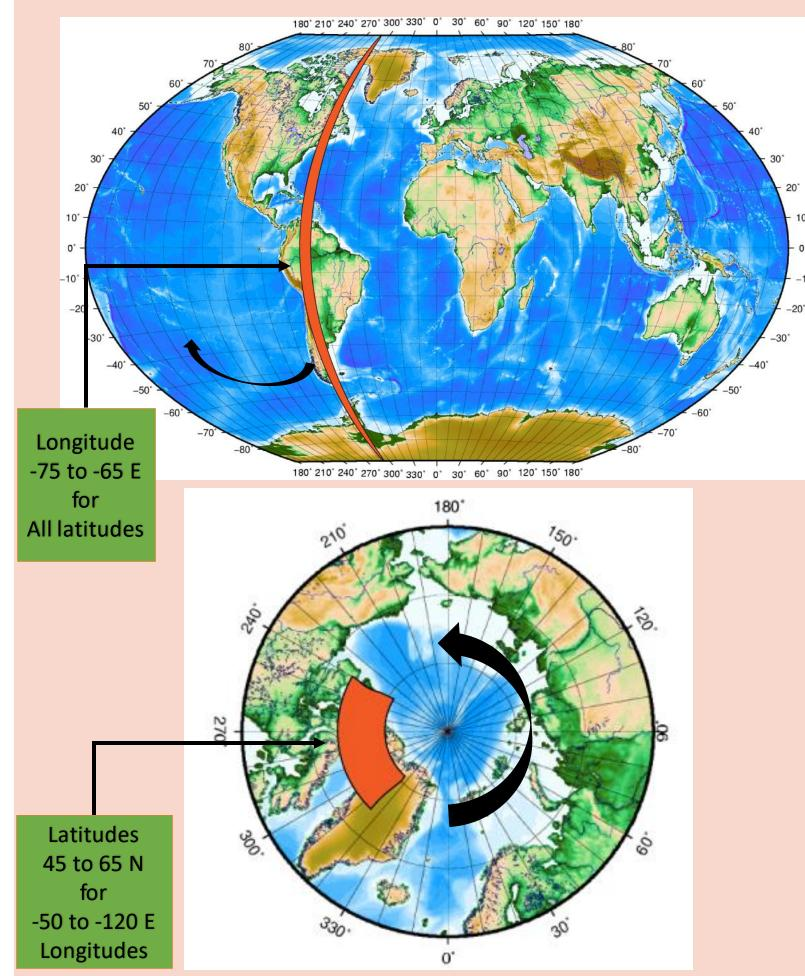
**TEC perturbation (dTEC)** Keogram maps were created in Geographic Coordinates for selected latitudes and longitudes (as shown in figure on the left) obtained by detrending TEC with a 30min running mean- for all links between a groundbased GNSS receiver and visible navigation
