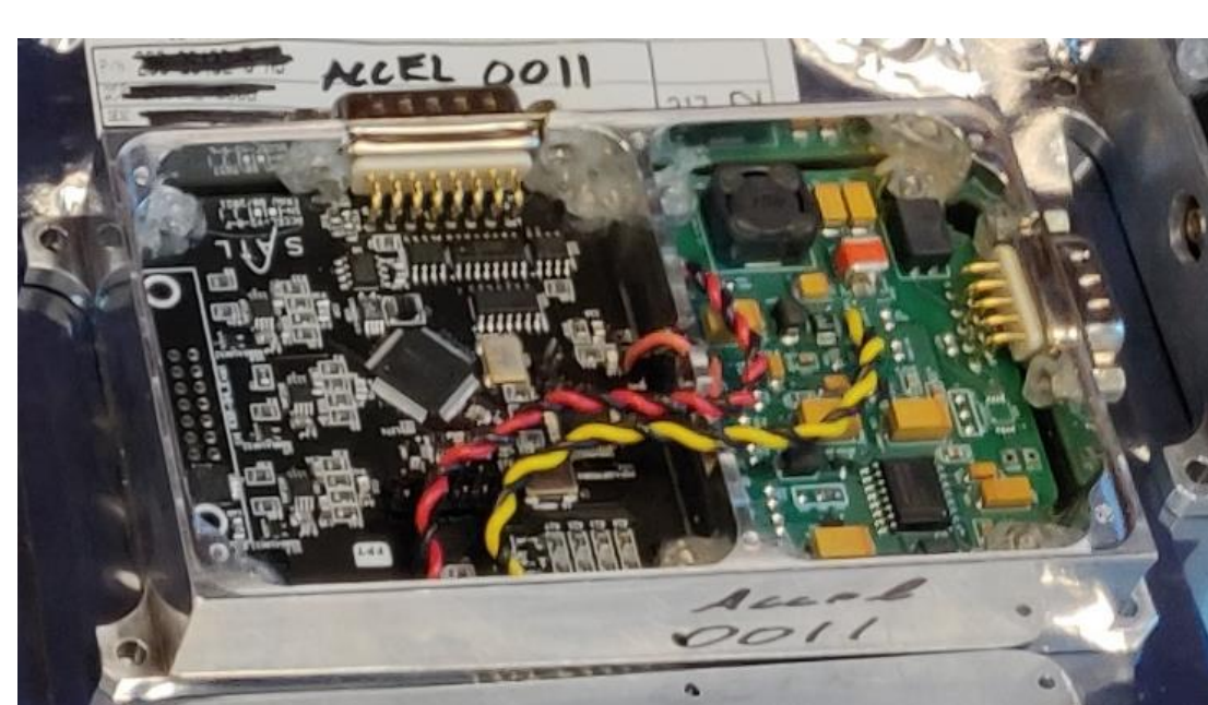
Main Payload Accelerometer Box
