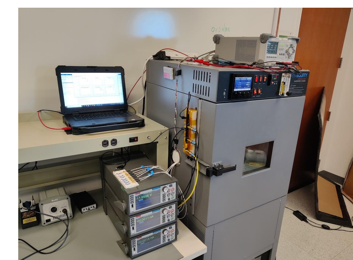
Figure 5: Image of the calibration setup in SAIL. Test Equity 115A shown on right. Left: 3 Keithley 2450 sourcemeters for simultaneous calibration.
