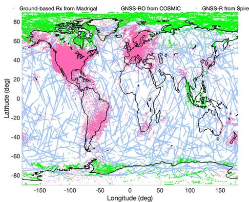
One day of TEC measurements from ground-based receivers from Madrigal (magenta), GNSS-RO from COSMIC (blue), and GNSS-R from Spire Global CubeSats (green).
