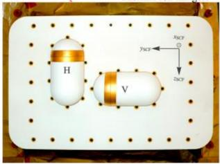
Fig 5.) TII sensor orientation on Swarm. One sensor is orientated in a horizontal direction and one in a vertical direction. Cross-track velocities obtained from only the horizontal sensor [3]
