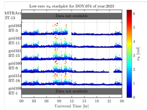
Fig 3.) Low-rate phase scintillation indices for each receiver at Poker Flat
