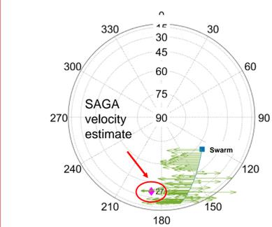
Fig 12.) Decomposition of velocities into cross-track direction shown on a sky plot
