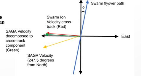
Fig 11.) Decomposing SAGA velocity to line up with Swarm velocity. Positive Velocity means Eastward
