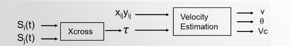
Fig 4.) Diagram of steps taken to find the velocity using SAGA
