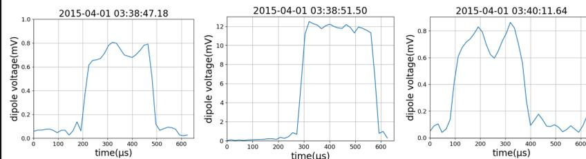
Fig 3; some random pulses. •Shortest interpulse period is around 1500 micro- seconds. And this value is not constant. •Beam switching period is 1 seconds. •Pulse width is 300 micro-seconds.
