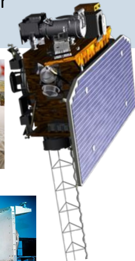
CCOR-1 integration onto GOES-U Image Credit: Lockheed Martin
