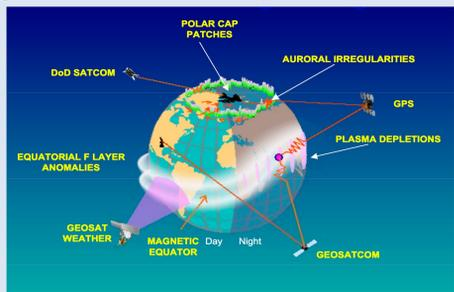
Figure 1. Schematic plot highlighting the ionospheric structures that can disrupt communication and navigation signals (From Basu, 2003). This proposal targets high-latitude irregularities and scintillations.
