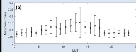
Figure 3: The average of each MLT hour of the maximum amplitude (a) and phase (b) scintillation that occurred in a 3-minute period centered on when a patch was observed.
