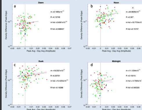
Figure 5: The density difference (peak - edge) as a function of peak average minus daily average amplitude scintillation for different MLT time periods
