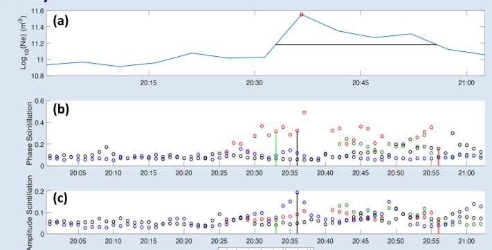
Figure 7: (a) Electron Density, (b) Phase, and (c) Amplitude Scintillation from several PRNs. In (a), the patch width is shown marked with a black horizontal line at 75% prominence with the red star marking the patch center. The green line marks the leading edge, the black line marks the center, and the red line marks the trailing edge in (b) and (c).
