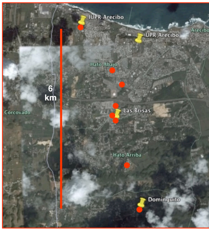
Figure 2: Google Earth image showing potential field sites (red dots) for eight receivers, in Puerto Rico near Arecibo Observatory, spread over a variety of linear north-south baselines ranging from 50 m to 6 km. These receiver locations were used to calculate the reconstructed image shown in figure 1.
