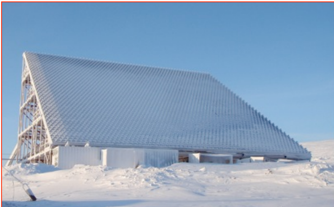
Resolute Bay (RISR-N): the latest phased array incoherent scatter radar observing the highest magnetic latitudes. Photo: Craig Heinselman
