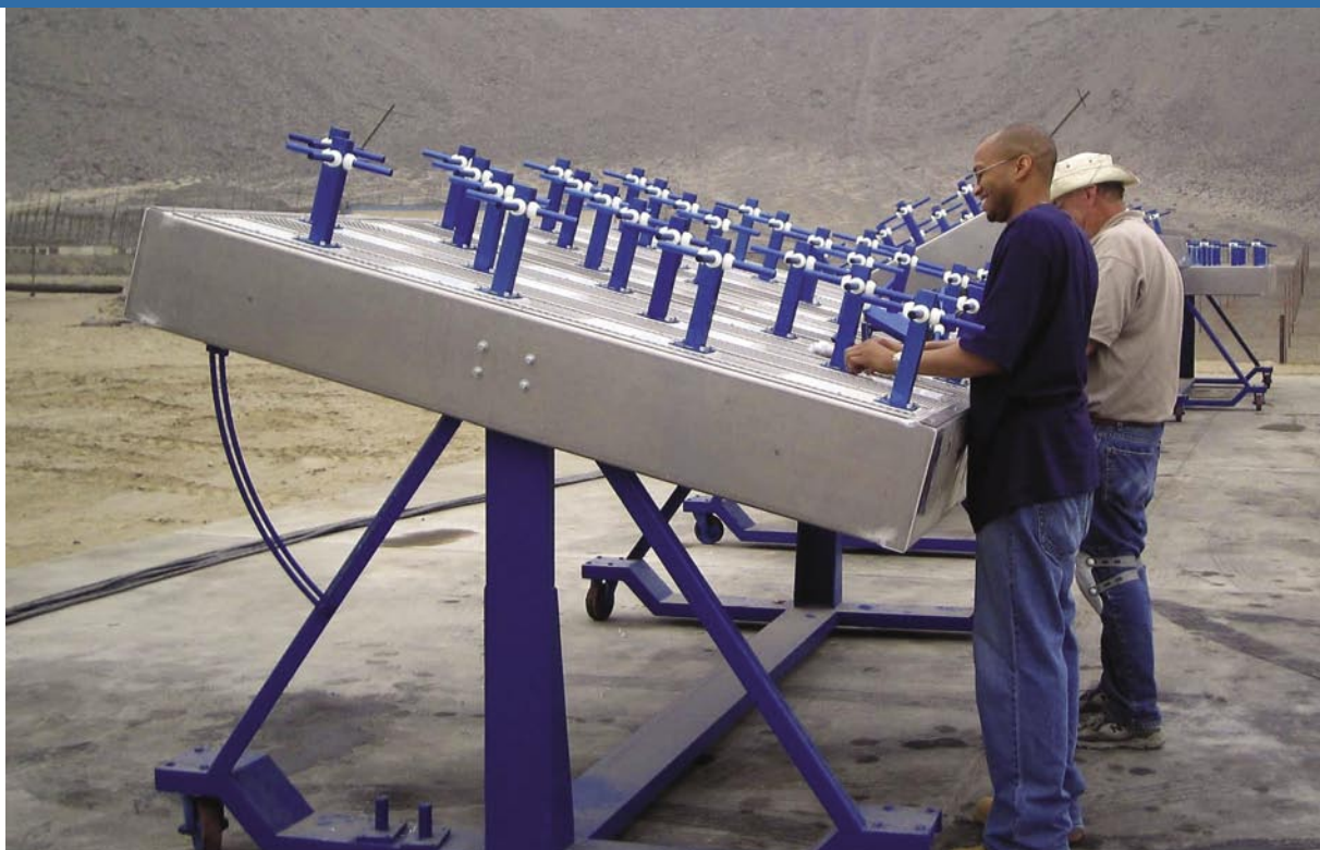
Assembling antennas onto a panel/cart at Jicamarca.
