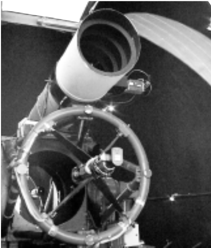
Figure 2. The dual telescope system housed at Firepond. The 1.2m primary can be seen in the bottom left corner, and the co-mounted and aligned 60cm telescope is contained within the white hood.
